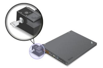
2. Press the eject button until the computer moves up. Then, grasp both sides, and remove the computer.
